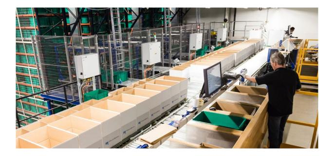
The picking storage solution for Wittusen & Jensen is based on three K.Store miniload cranes with multi-retrievers for storage and outfeed of items of various dimensions at the same time.
