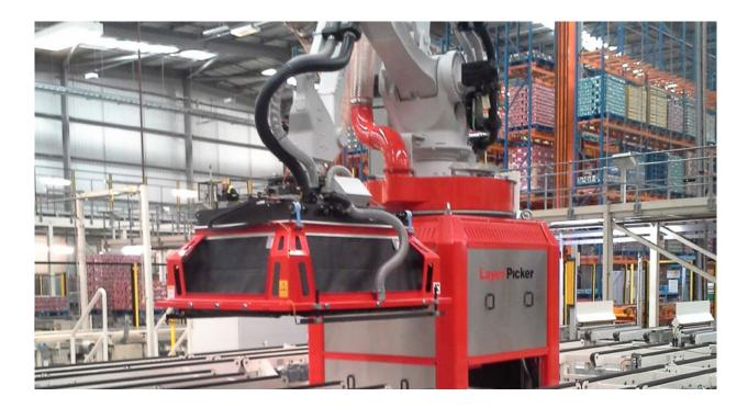
Kraft Heinz wanted a significant increase in the amount of pallet layers being picked automatically without making changes in the existing product configuration. This was achieved with the installation of a K.Handle Layer Picker® Flex-R from Körber.
