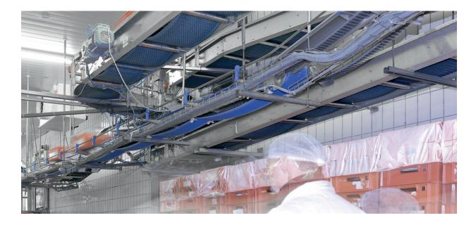
With a multi-stage retrofit project, Körber is bringing Wilhelm Brandenburg's intralogistics up to the current state of the art. An efficient modernization solution was implemented, under the restrictive conditions of hygiene and cooling regulations for temperaturecontrolled fresh produce logistics, as well as tight time frames for implementation during ongoing production
